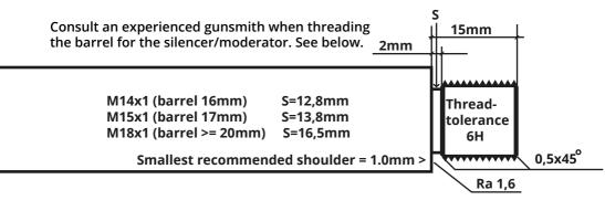
Thread and bore in center and in line with the silencer.
